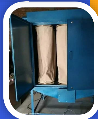
Dust Collector Machine
