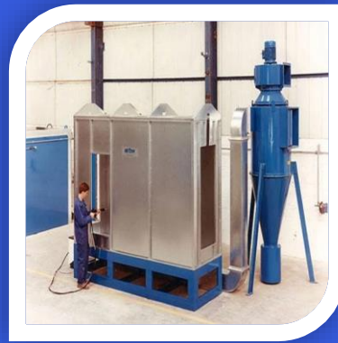
WOOD GRAIN SUBLIMATION PLANT FOR ALMUNIU PROFILE
